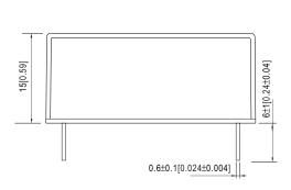
Case No.IRM02 Unit:mm[inch] Tolerance:±0.5[±0.02] unless otherwise specified
