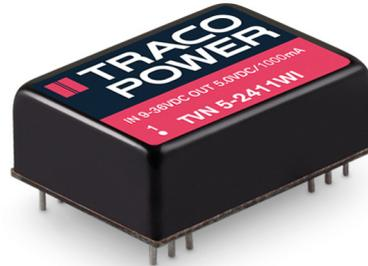
The TVN 5WI series is a ultra low ripple and noise 5 Watt DC/DC converter in six side shielded metal package. The conducted noise complies with EN 55032 class B and makes this converters the ideal solution for audio, measurement and detection circuits.
