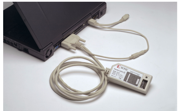
Figure 7: Laptop PC4 Cable Connection
