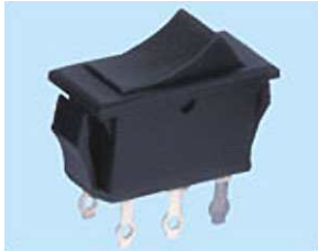
RS2025C ON-ON RS2035C ON-OFF-ON 6 A 125 VAC; 3 A 250 VAC DPDT 6P
