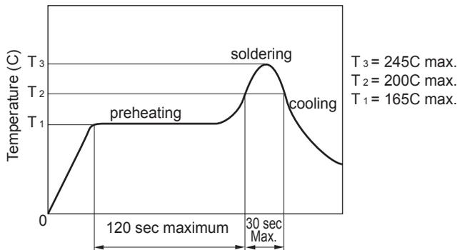
VPS (Vapor Phase Soldering)
