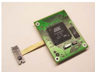
Figure 1. FingerChip Biometric Module AT77SM0101BCB02VKE
