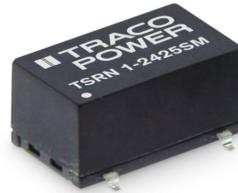
The new TSRN-1SM series are step-down non-isolated switching regulators in compact SMD package. They are an ideal solution to replace inefficient linear regulators. The high efficiency up to 95% allows full load operation up to  $+55^{\circ}\text{C}$  ( $+85^{\circ}\text{C}$  with derating) ambient temperature without the need of forced air cooling.
