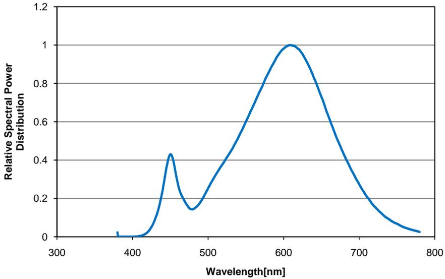
Fig 2. Relative Spectral Distribution vs. Wavelength Characteristic – E
