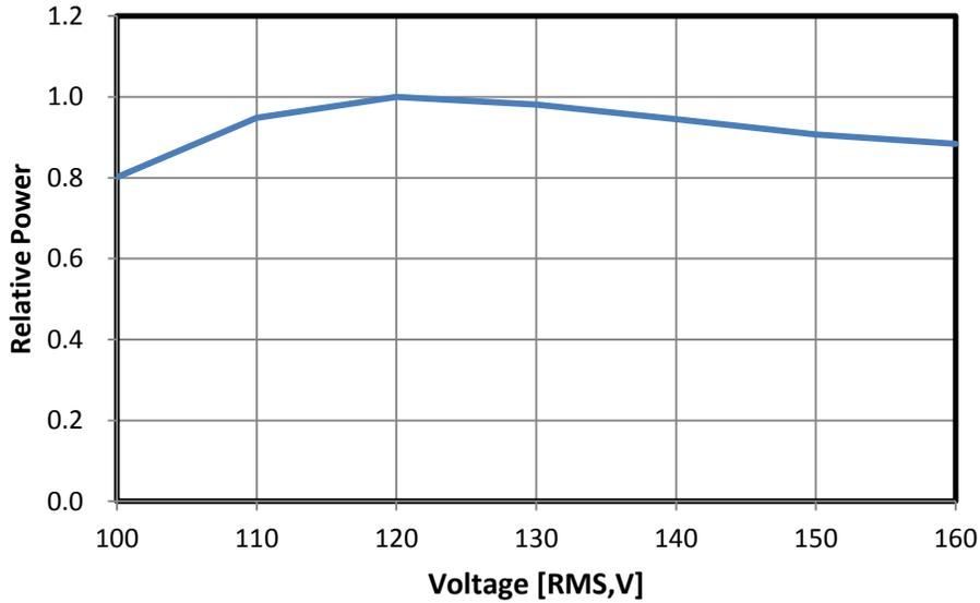
**Fig 5. Relative Power Distribution vs. Voltage,  $T_a=25^{\circ}\text{C}$ , 220V**
