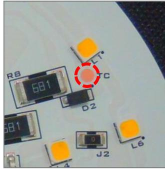
The Acrich3 module is recommended to keep the junction temperature under maximum junction temperature spec. (Table 5)
