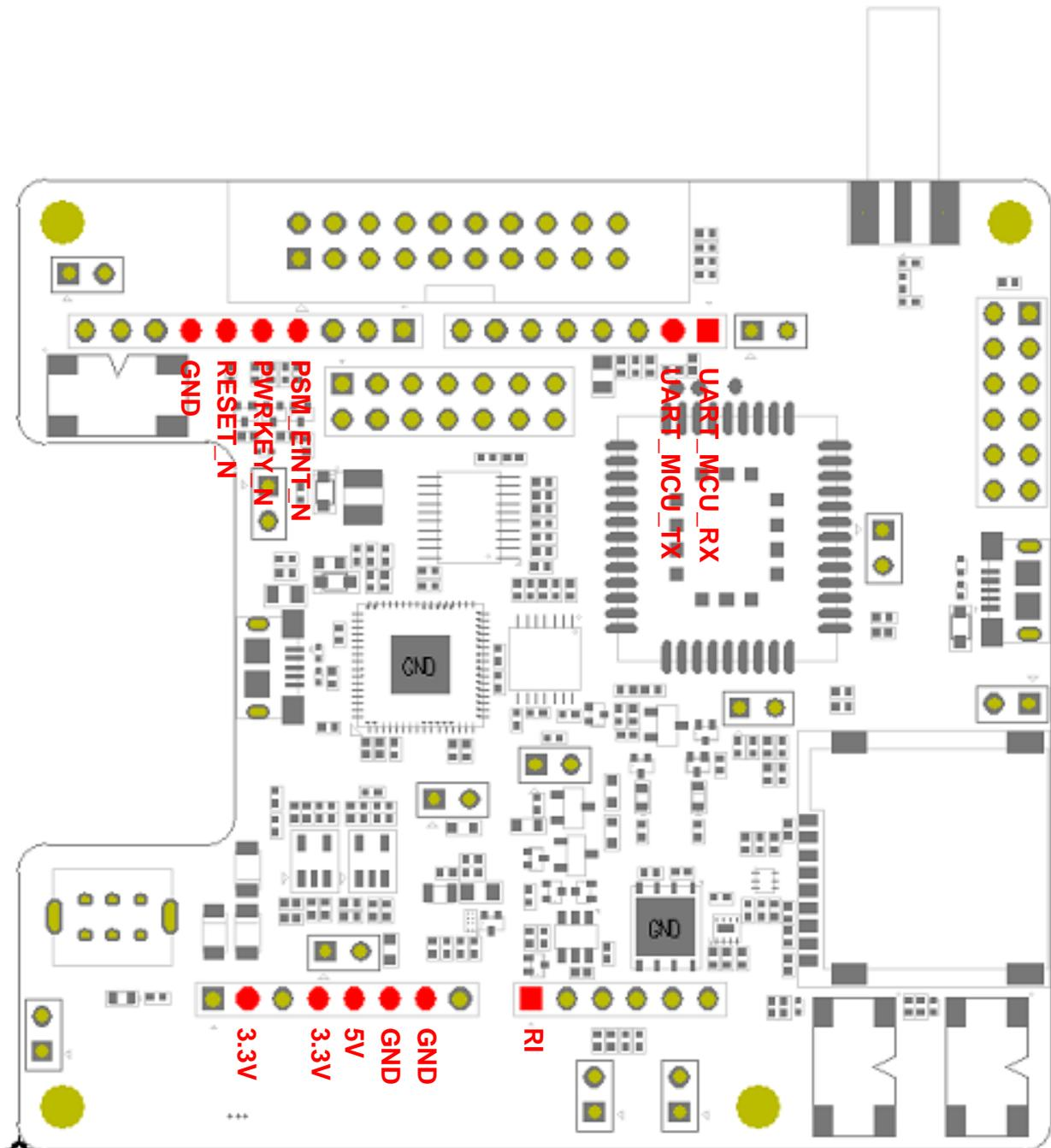
Figure 3: Arduino Interface Definition
