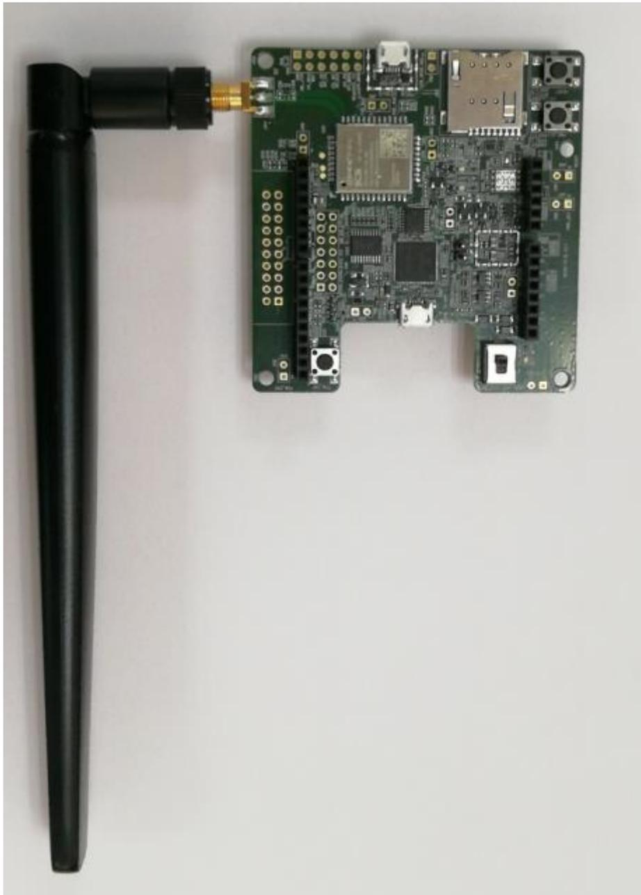
Figure 14: BC66-TE-B Kit Assembly
