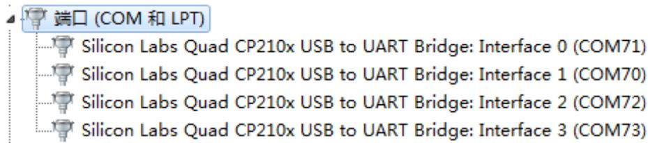
Figure 5: UART Ports Displayed on PC
