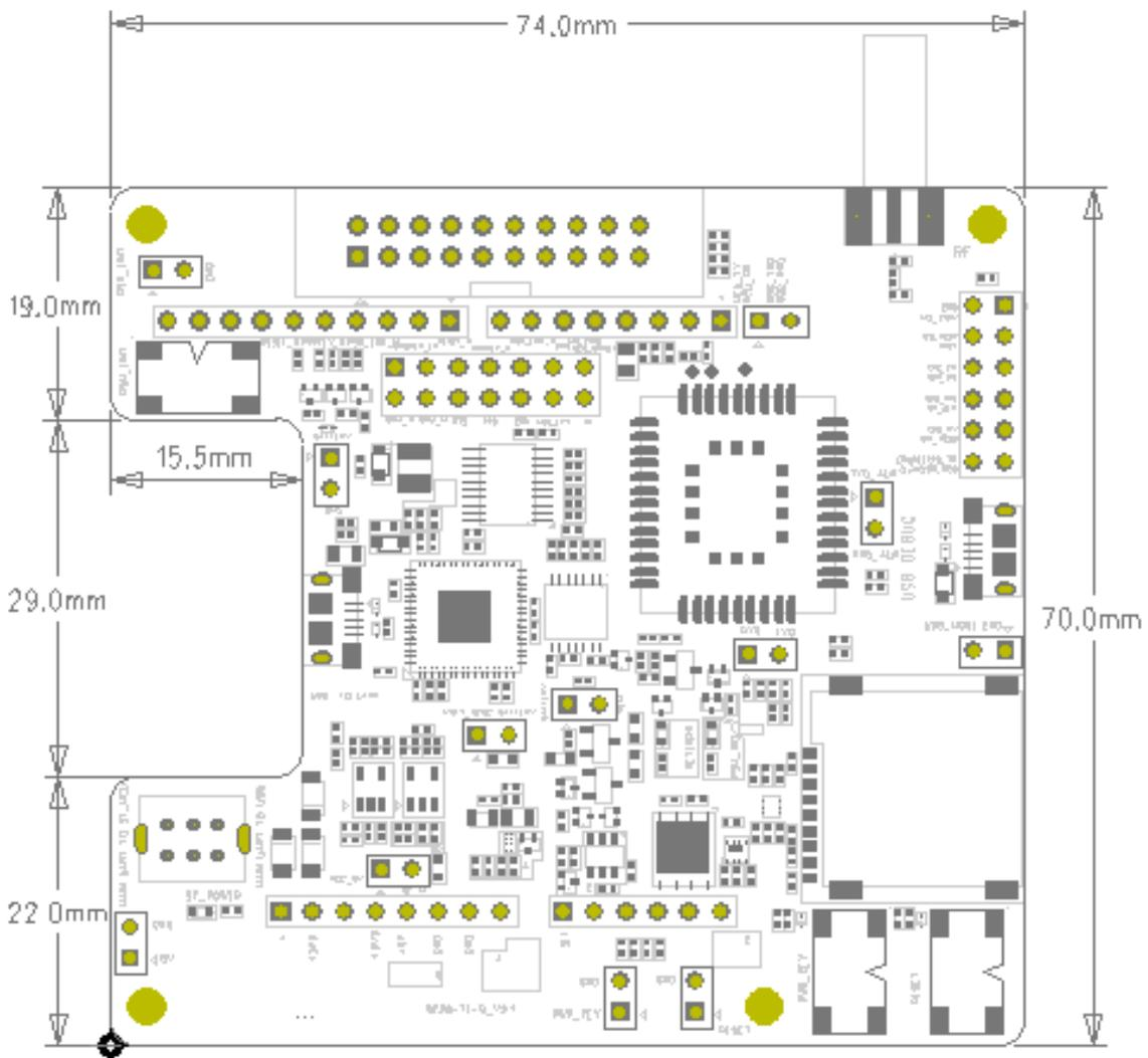
Figure 11: Dimensions of BC66-TE-B (Top View)
