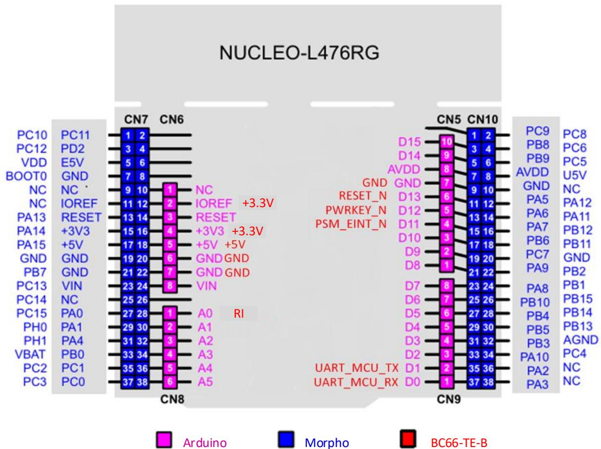
Figure 10: Pin Connection between BC66-TE-B and STM32-L476RG MCU
