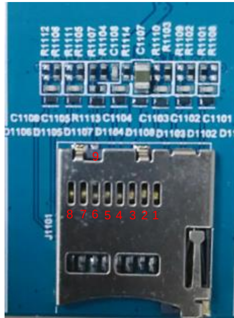
Figure 38: Pin Assignment of SD Card Interface
