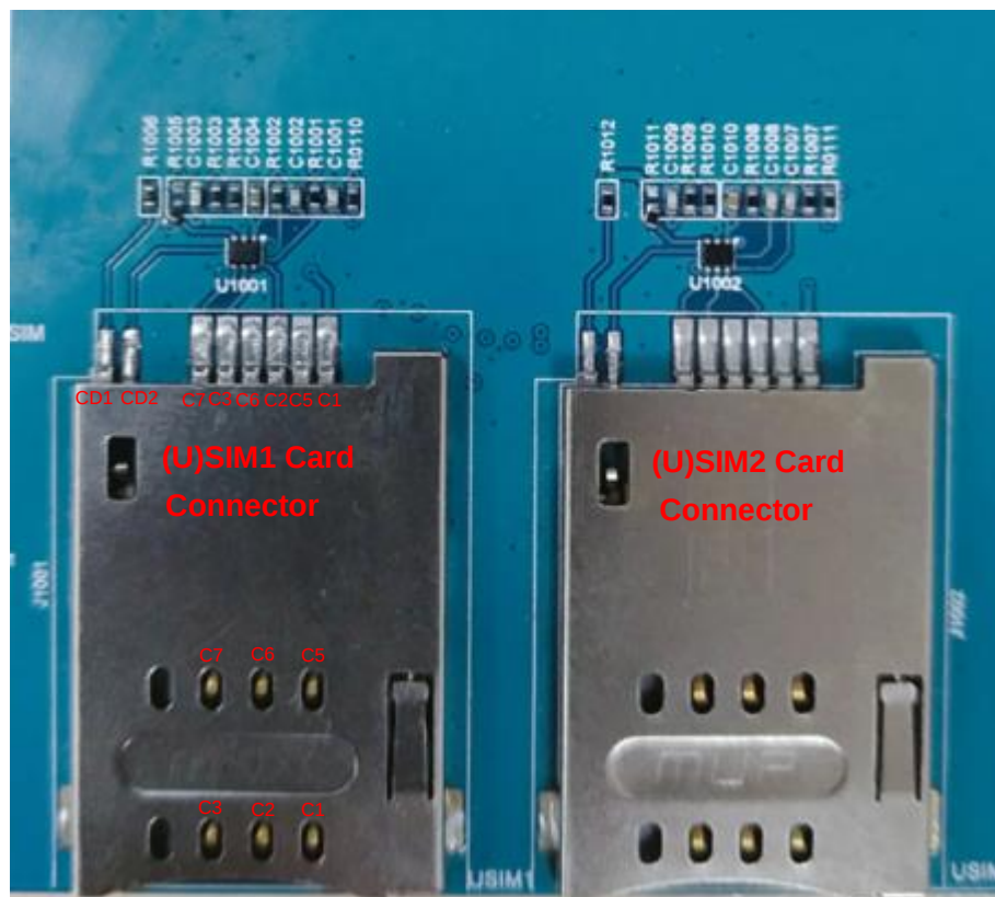
Figure 34: Pin Assignment of (U)SIM1 Card Connector
