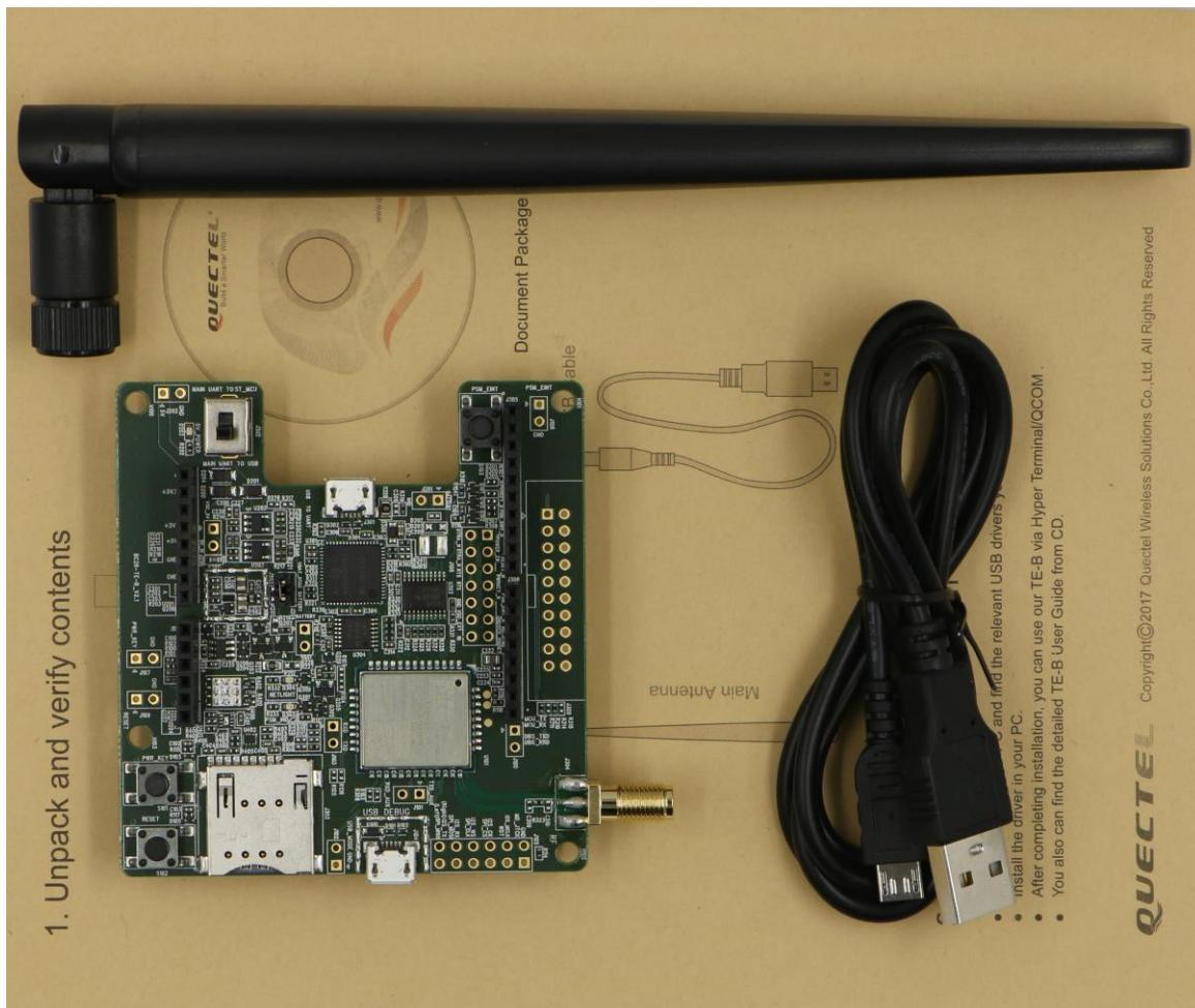
Figure 15: BC66-NA-TE-B and the Accessories
