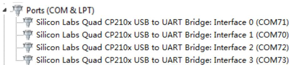
Figure 5: UART Ports Displayed on PC
