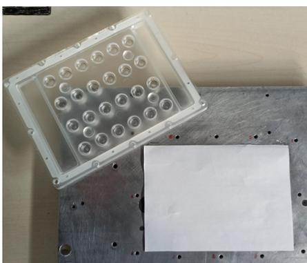
As shown in the photo, the test paper sheet is completely dry after disassembling the system.
