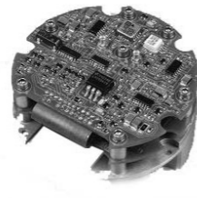
SAU Electronics Assembly for ground to air missile application
