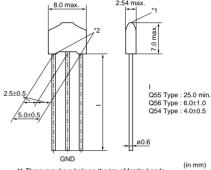
\*1 There may be a hole on the top of ferrite beads, which cause no characteristics deterioration.
