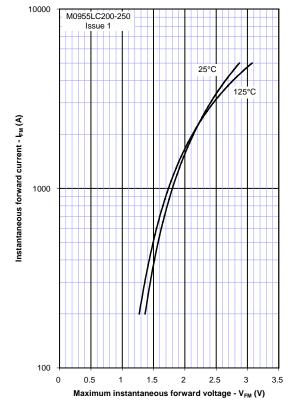
Figure 1 – Forward characteristics of Limit device
