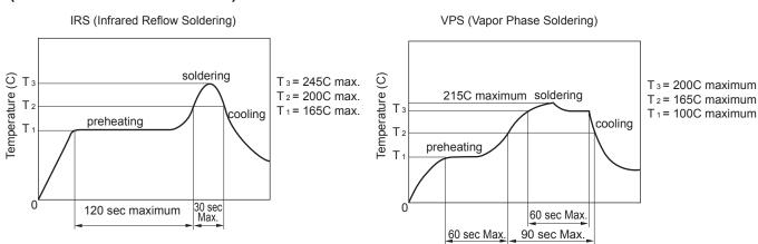
1. Temperature profiles show the temperature of PC board surface.
