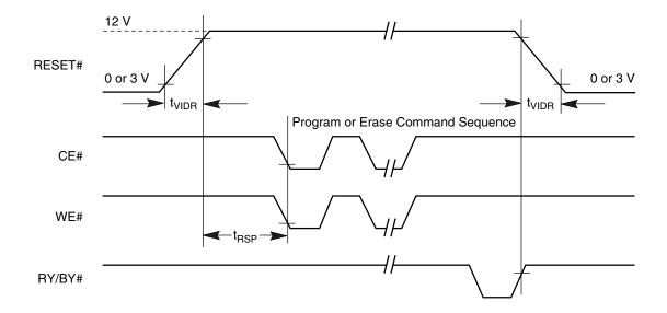
Figure 22. Temporary Sector Unprotect Timing Diagram
