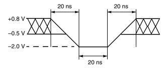
Figure 7. Maximum Negative Overshoot Waveform
