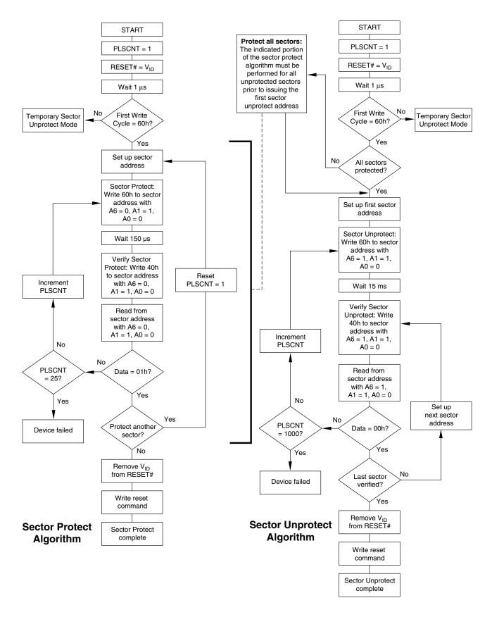
Figure 1. In-System Sector Protect/Unprotect Algorithms
