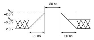
Figure 8. Maximum Positive Overshoot Waveform
