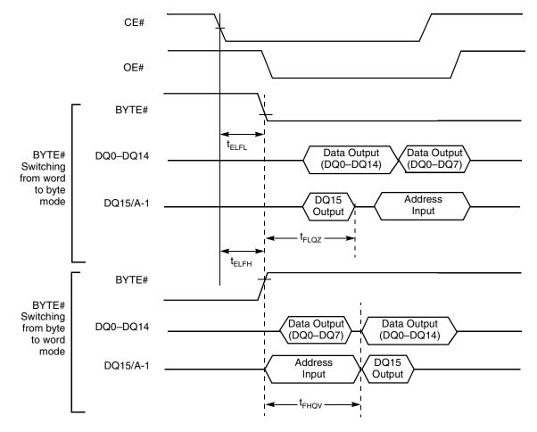
Figure 15. BYTE# Timings for Read Operations
