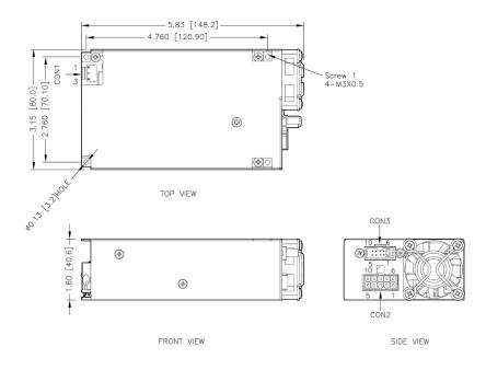
FAN dimension: 40×40×10mm Air flow: 9.5 CFM The fan's durability is lower compared to the power supply and has only 2 years warranty.
