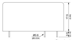
Dimensions in mm (inch) Tolerances:  $x.x \pm 0.5 (\pm 0.02)$
