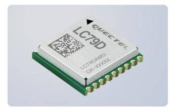
LC79D is a high performance GNSS module supporting multi-constellation GNSS and dual GNSS bands. It can acquire and track GPS, GLONASS, IRNSS, BeiDou, Galileo and QZSS signals. The module can work at L1 and L5 Bands for GPS and GALILEO satellites.
