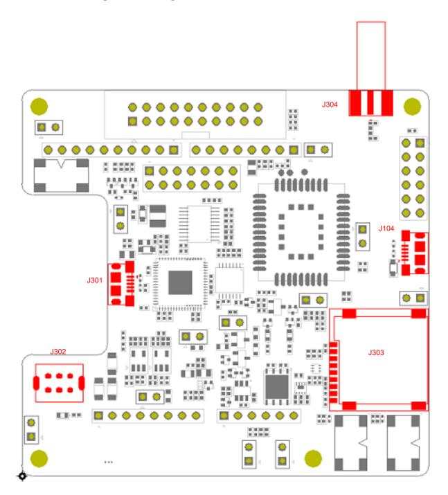
Figure 4: Interface Diagram of Using BC66-TE-B Alone
