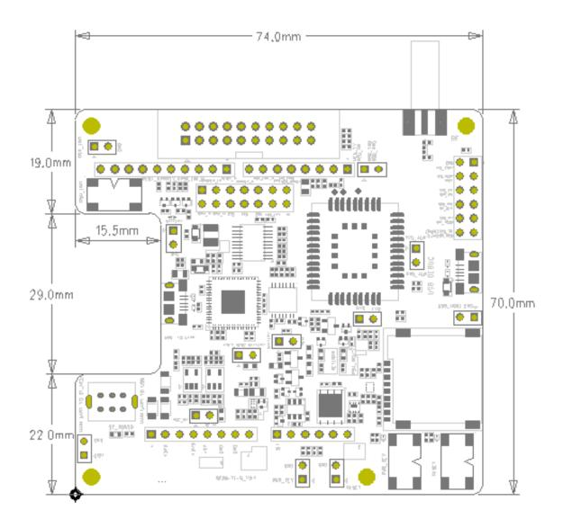
Figure 11: Dimensions of BC66-TE-B (Top View)
