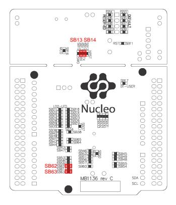
Figure 8: STM32 Nucleo-64 Board Modification Diagram (Bottom View)
