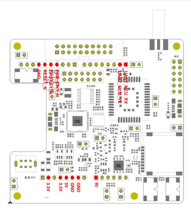
**Figure 3: Arduino Interface Definition**
