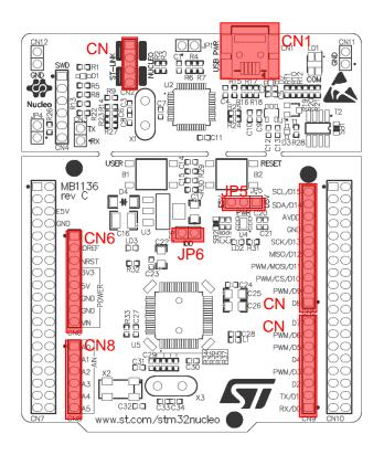
Figure 7: STM32 Nucleo-64 Board Interface Diagram (Top View)
