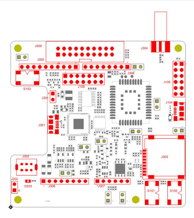
Figure 2: Interface Distribution Diagram of BC66-TE-B
