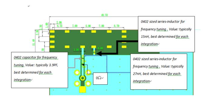
The antenna requires a matching circuit that must be optimized for each product. The matching circuit will require up to six components and the following circuit should be designed into the host PCB. Not all components may be required but should be included as a precaution. The matching network must be placed close to the antenna feed to ensure it is more effective in tuning the antenna.
