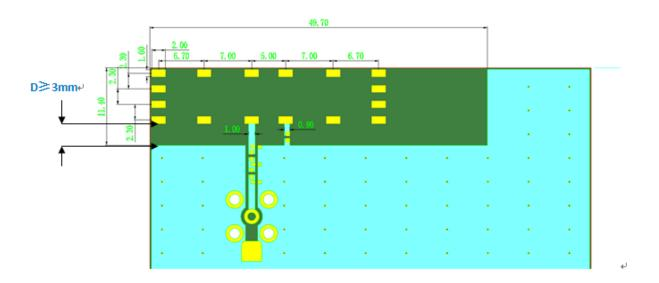
**Gap D** is required from the edge of the antenna to the ground plane. This should be maintained along the edge of the antenna placement, **minimum value is 3 mm**.
