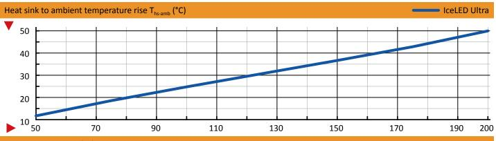
Dissipated Power Pd(W)
