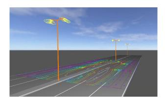
Street Type Pole to pole distance: 40m Pole height: 15m Light overhang: 1m Boom angle: 10° Road width: 16m
