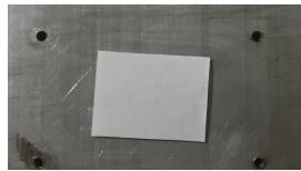
As shown in the photo, the test paper sheet is completely dry after disassembling the system.
