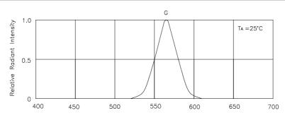
wavelength  $\lambda$  (nm) RELATIVE INTENSITY Vs. WAVELENGTH
