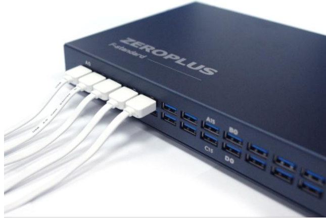
Figure 2-3 Test cables connected to the LAP-F1
