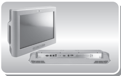
▲ Slim design with PCI or PCIe expansion and multiple I/O interface
