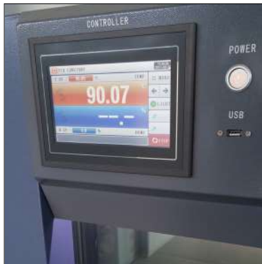
Temperature set in the climatic chamber
