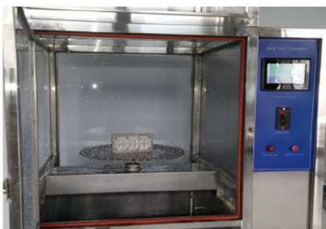
Testing under water jet
