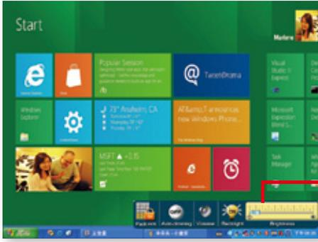
IEI patented system software utility allows users to adjust system settings through the software interface in Windows environment instead of pressing the membrane keypad below the front panel.
