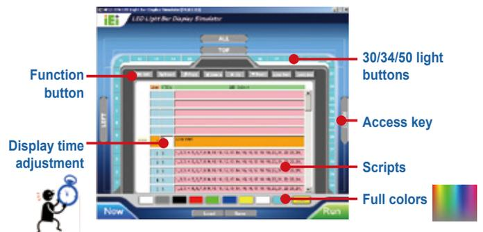
Support LED Light Bar control API for the customer to suit their own software program. Light bar signal are correspond to the light button. User can customize their own light patterns for different conditions.
