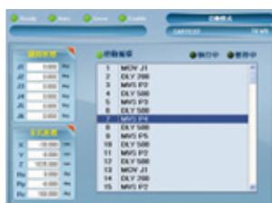
Run the programmed commands automatically. The cyclic operation mode is also supported.
