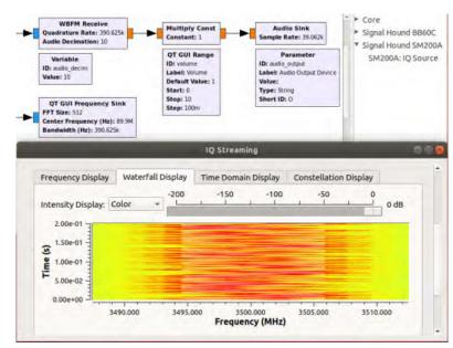
The GNU Radio application running the SM200B analyzer as a flowgraph block.
