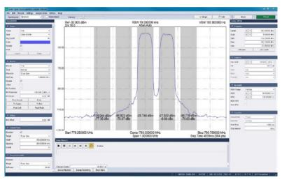
Adjacent Channel Power Ratio (ACPR) measurements.
