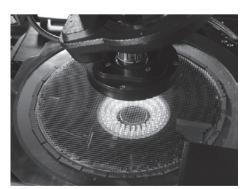
Chroma 7940 wafer inspection system is an automatic inspection system for after-dicing wafer chip. The appearance defects of wafer chip are clearly conspicuous by using advanced illumination technology. Illumination and camera acquisition mode can be adjusted for various wafer chip, like LED, laser diodes and photo diodes.
