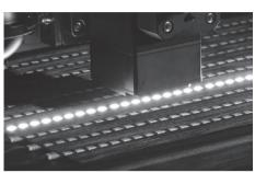
CIE127 Condition B measurement Module
