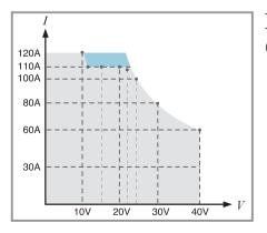
The blue area is over specification due to low voltage (<22V) & high current output(>110A). The following is operation power envelope :
