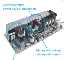
Secondary side voltage Secondary side current Multi-channel Data Logger
