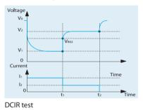
**Electrical Double Layer Capacitor Test**
