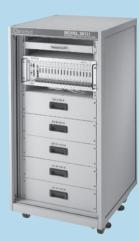
**OLED Lifetime Test System**
