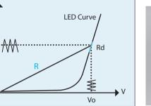
Figure 1 LED V-I Characteristics
