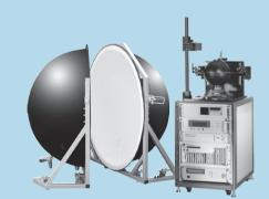
LED Lighting Test System (For Laboratory)
