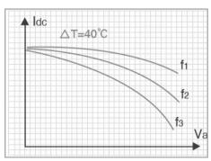
Load Current (ldc) and AC Voltage (Vac) Curve
