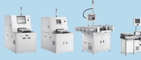
OCV/ACR Test Equipment Barcode Binding Equipment Rework Sorter
