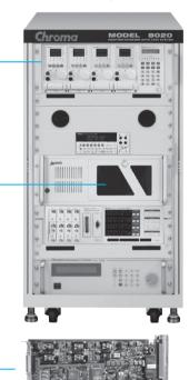
The 84903 Control Card is applied to verify Quick Charge 2.0 charger.
