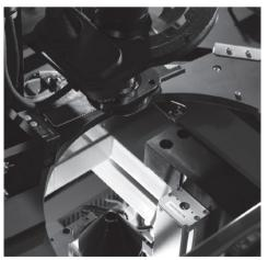
Chroma 7936 double sided wafer inspection system is an automatic inspection system for afterdicing wafer chip. It can do double side inspection simultaneously. The appearance defects of wafer chip are clearly conspicuous by using advanced illumination technology. Illumination and camera acquisition mode can be adjusted for various wafer process, like vertical chip or flip chip.
