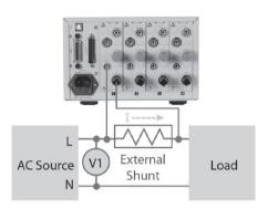
66203/66204 Power Meters support external shunt function for high current (>20A) measurement application.
