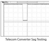
Sag Testing Output Voltage
