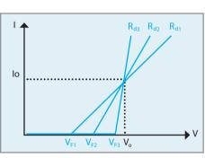
Figure 5 - Simulate different characteristic of LEDs
