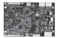
A270148 eDP Bist module can provides the DPCD control signal and power for panel into BIST mode, integrate with Chroma Aging system can provide a complete eDP panel aging test solution.
